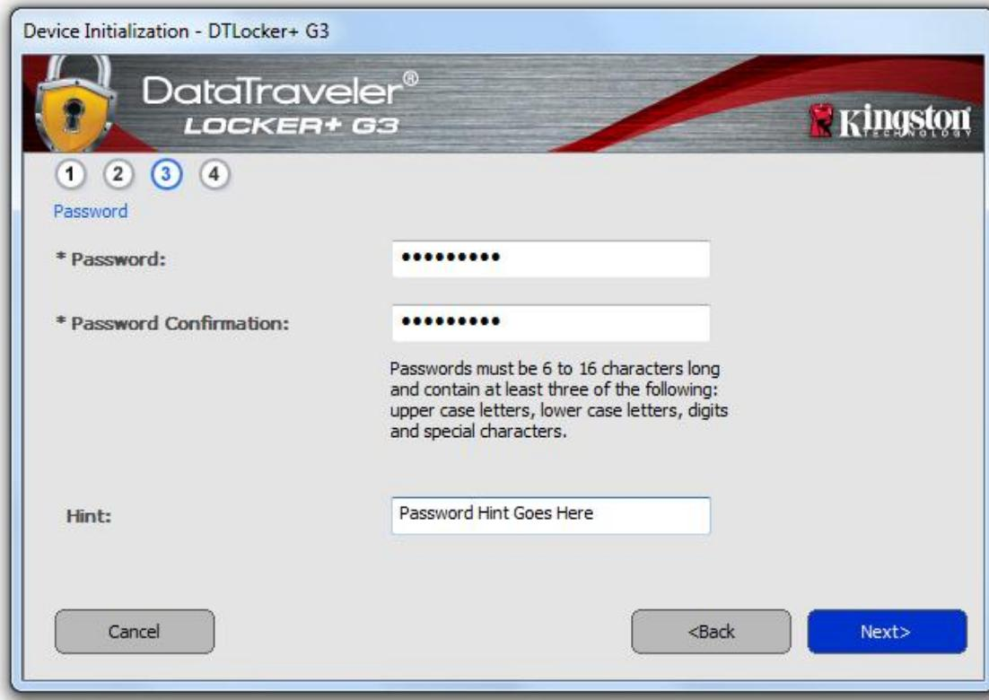
**Figure 3.3 – Password Setup**
